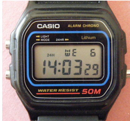
Figure 52: Casio Watch LCD Display (Creative Commons: Ricce)
