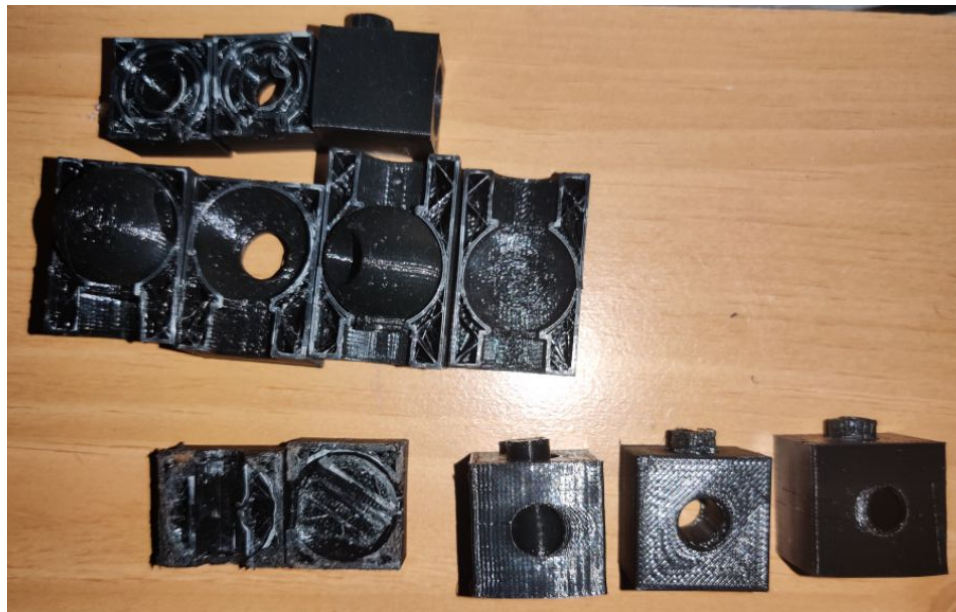
Figure 72: Iterative Design of Vent Ball Valves
